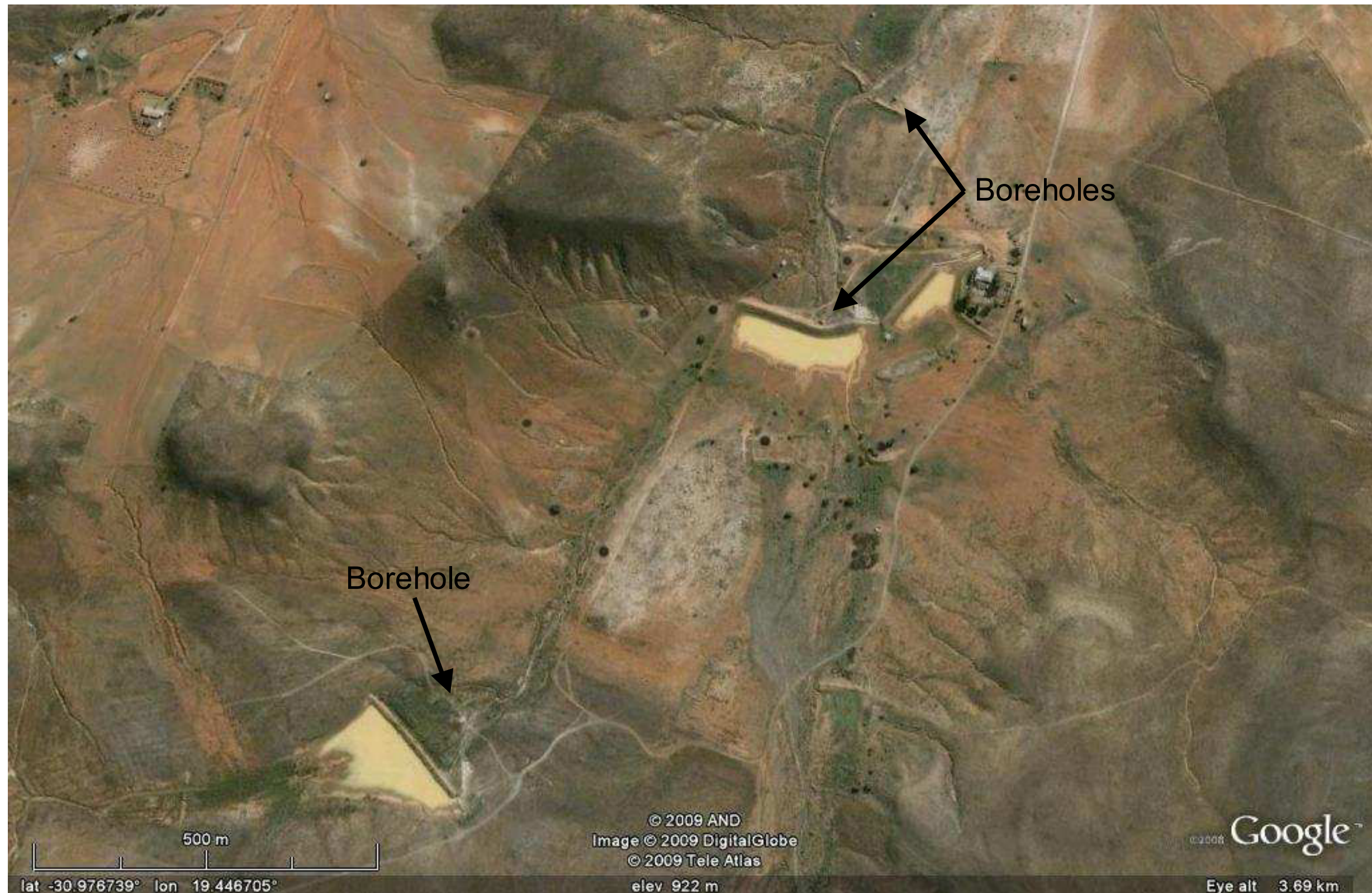
FIGURE 10 Loeriesfontein boreholes located below earth dam walls.
