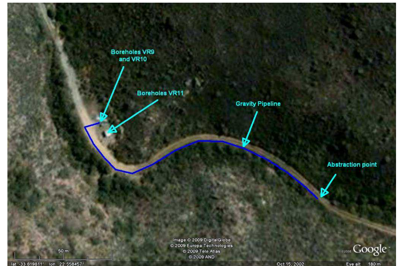
Figure A4.6 Layout of proposed gravity pipeline to injection boreholes VR 9 and VR10
