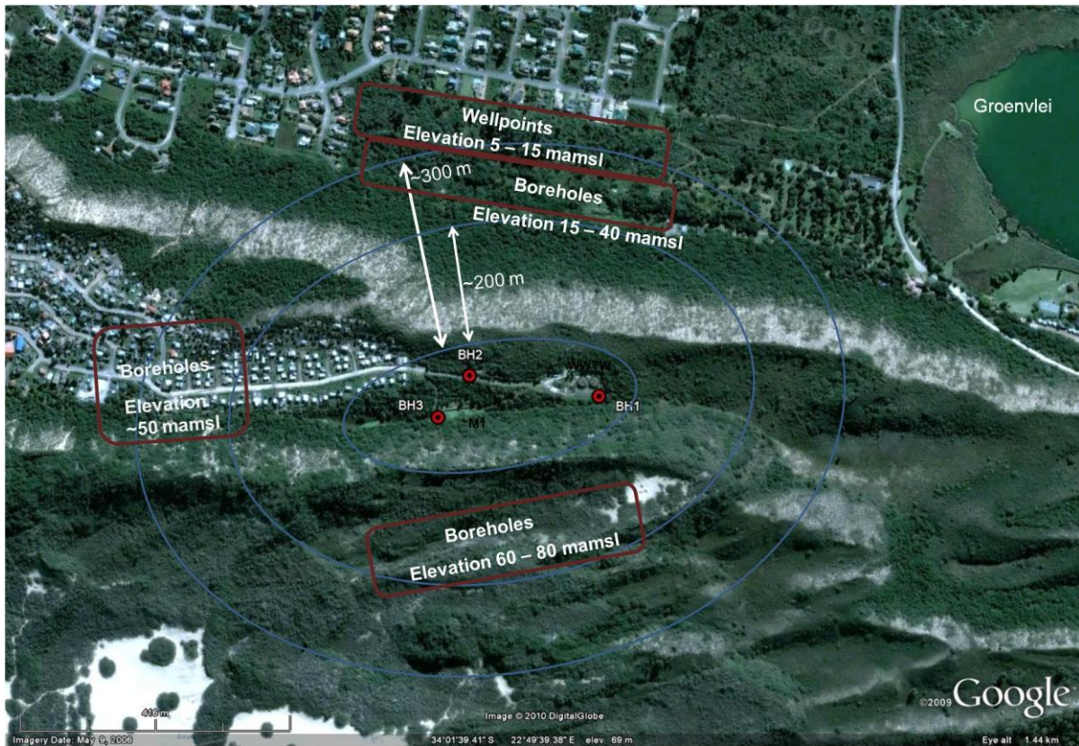
FIGURE 4.6 POSSIBLE LOCATIONS OF ABSTRACTION SITES TO INTERCEPT THE TREATED WASTE WATER (GOOGLE EARTH, 2010)
