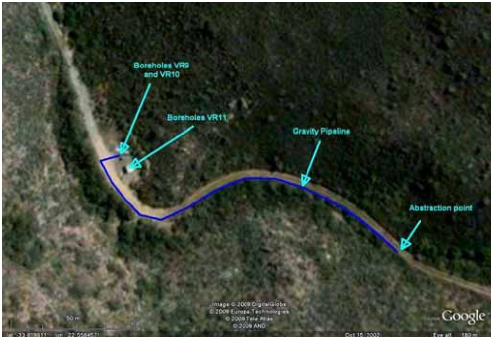
FIGURE 7.2 THE PROPOSED INFRASTRUCTURE TO TEST AR IN THE UPPER-MOST PART OF THE VERMAAKS RIVER WELLFIELD (GOOGLE EARTH, 2010)
